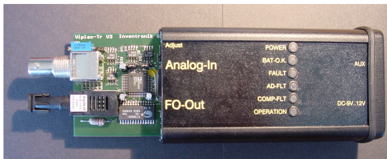
Figure 3: Disassembly of the transmitter PCB to the left side!
