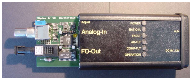
figure 5: Disassembly of the transmitter PCB to the left side!
