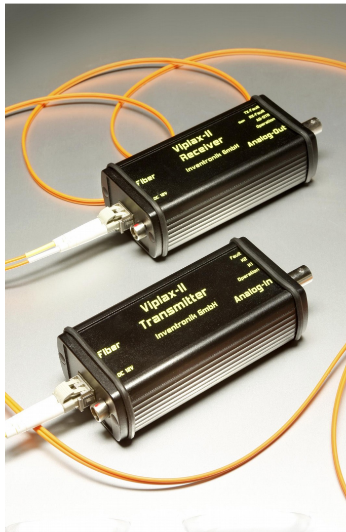
Figure 1: Analog transmission system in the handheld form factor
