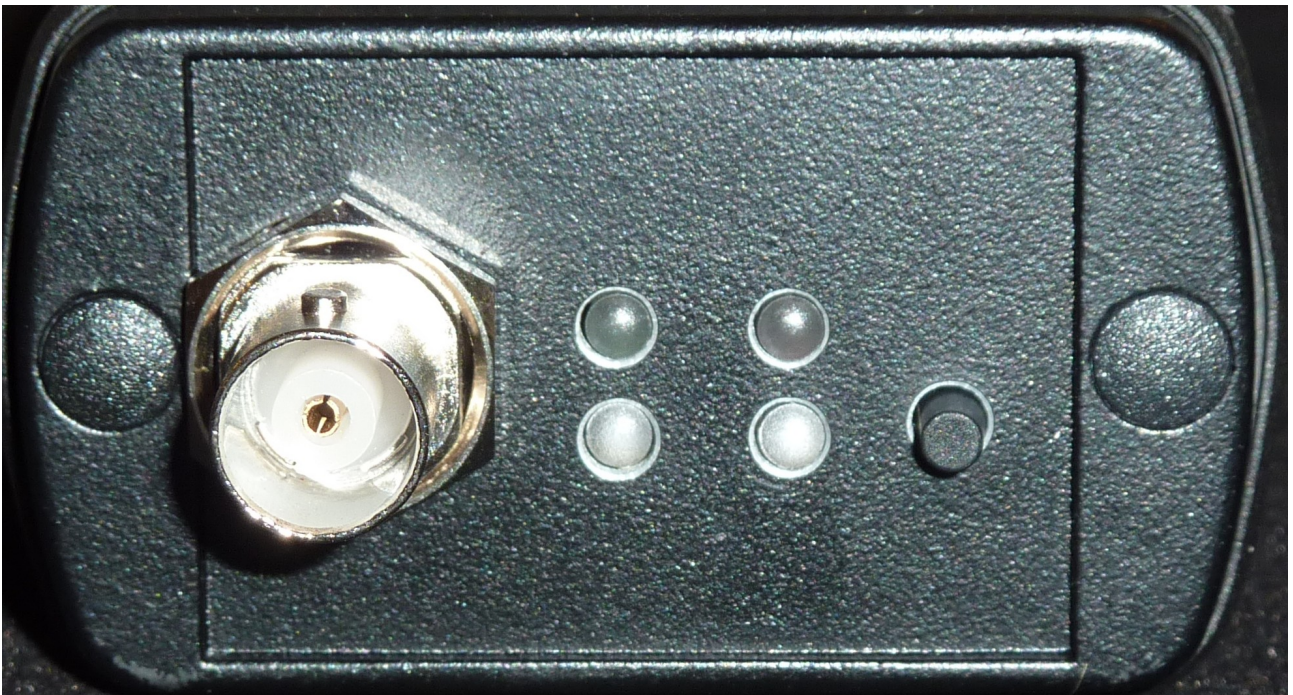
Figure 2: Status LEDs of a Viplax-IIA Handheld Unit
